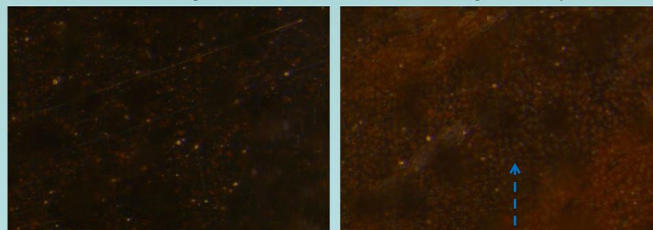
Micropores (1µm-10µm) due to the volatile products (H<sub>2</sub>, N<sub>2</sub>, CO<sub>2</sub>)
