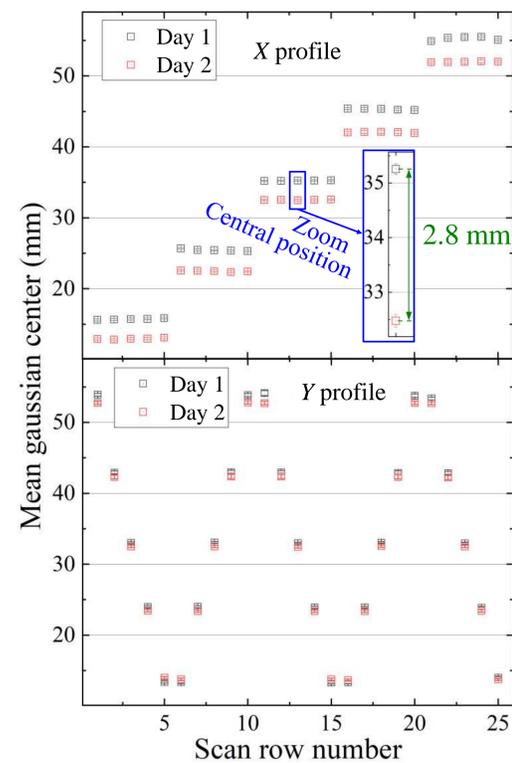
• A 2.8 mm shift in the  $X$  profile position was observed → likely due to a difference in the manual positioning of the setup, following the replacement of the anodes.
