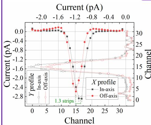
• Off-axis design shows lower current → linked to electrode geometry. Can be corrected via calibration, with no impact on performance.
